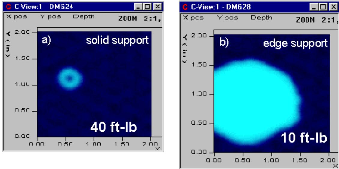
Figure 4. Through-transmission C-Scans of (a) solid- and (b) edge-supported coupons of low-porosity, impact damaged with energy of 40 and 10 ft-lb, respectively.
