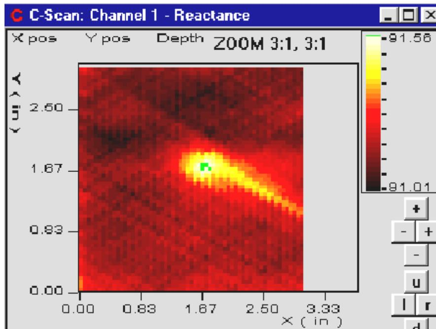
Figure 6. Eddy current scan image of the coupon impact-damaged with edge support and energy level of 40 ft-lb.
