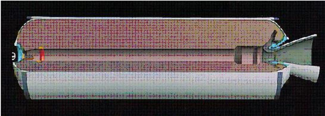
Figure 1. Typical solid rocket motor (SRM).
