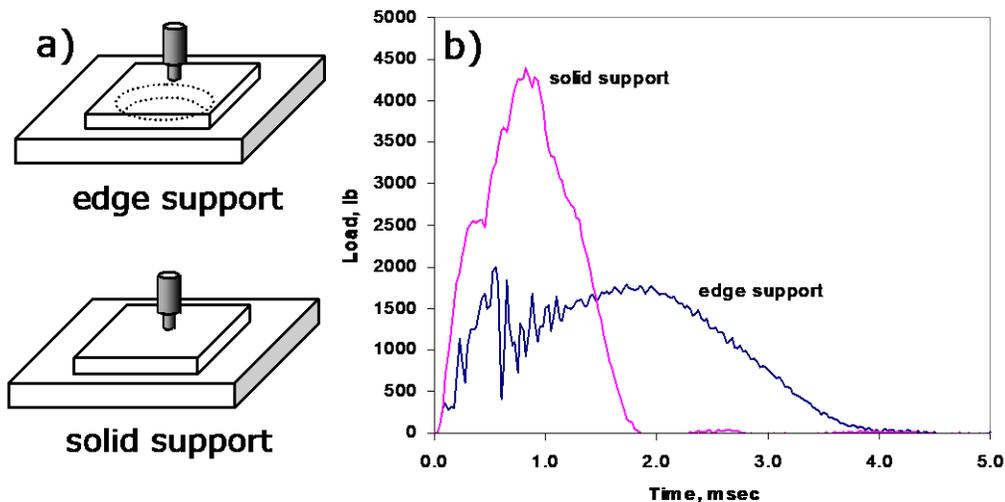
Figure 2. (a) Solid and edge support conditions; (b) Typical impulse curves for solid- and edge-supported coupons.
