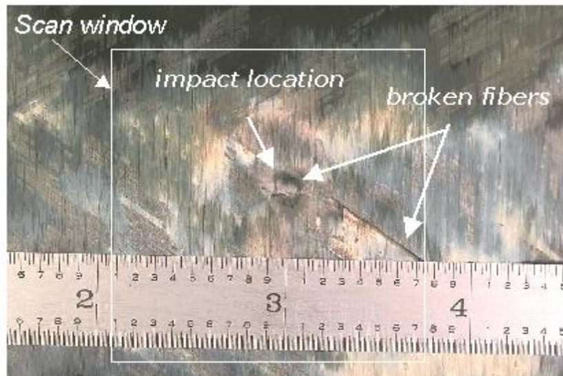
Figure 7. Photograph of deplied 4<sup>th</sup> layer ( $90^\circ$  direction) of the coupon impact-damaged with edge support and energy level of 40 ft-lb
