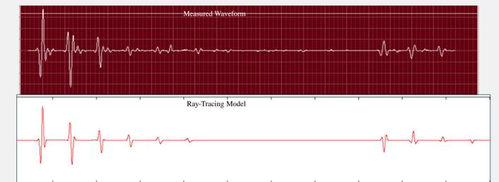
Figure 5. Comparison of Measured Waveform and Model Calculation
