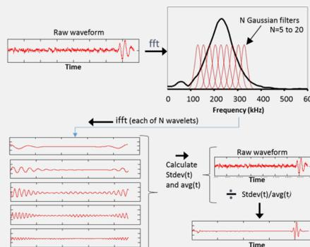
Figure 2. Graphical Representation of Split Spectrum Processing Method
