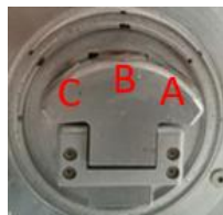
FIGURE 6. Sensor assignments on eddy current probe.
